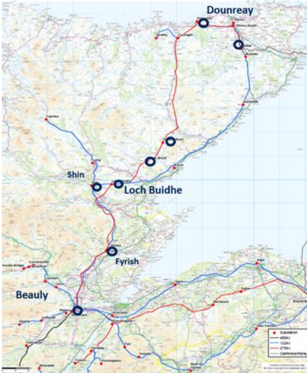
Figure 1: Map showing the existing Beauly to Loch Buidhe to Dounreay 275kV OHL
