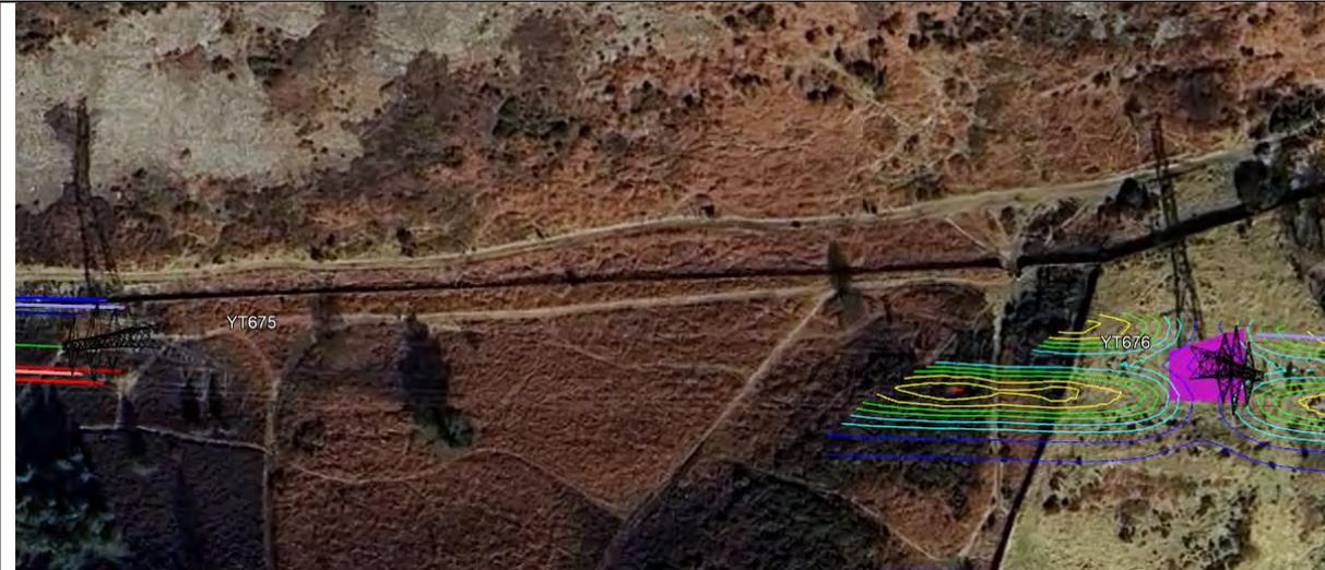
Figure 10 Electric Field Contours (kV/m) for span 675 to 676
