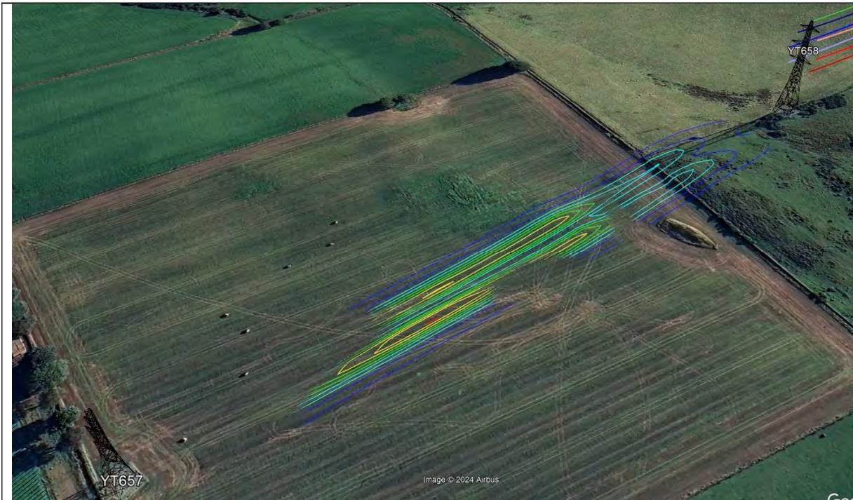
Figure 8 Electric Field Contours (kV/m) for span 657 to 658
