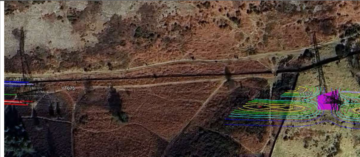
Figure 10 Electric Field Contours (kV/m) for span 675 to 676
