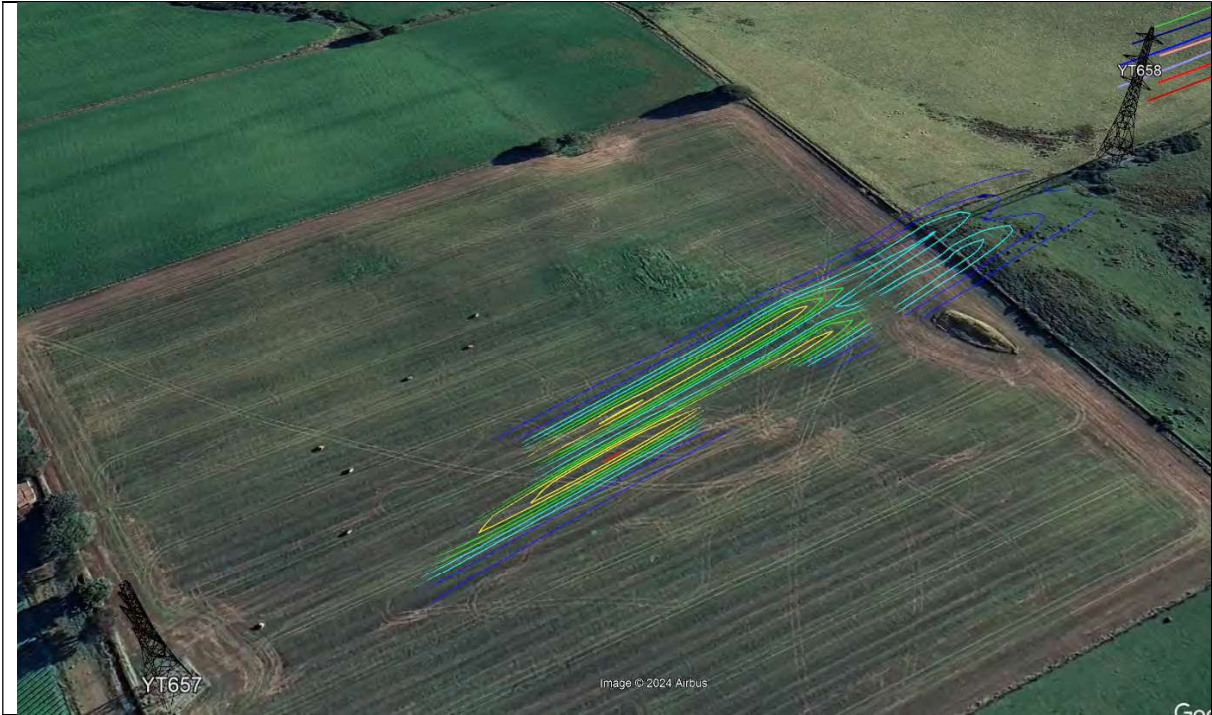
Figure 8 Electric Field Contours (kV/m) for span 657 to 658
