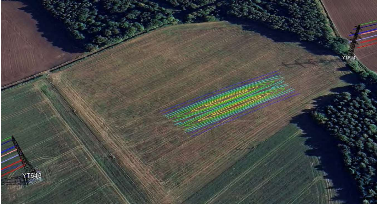
Figure 4 Electric Field Contours (kV/m) for span 643 to 644
