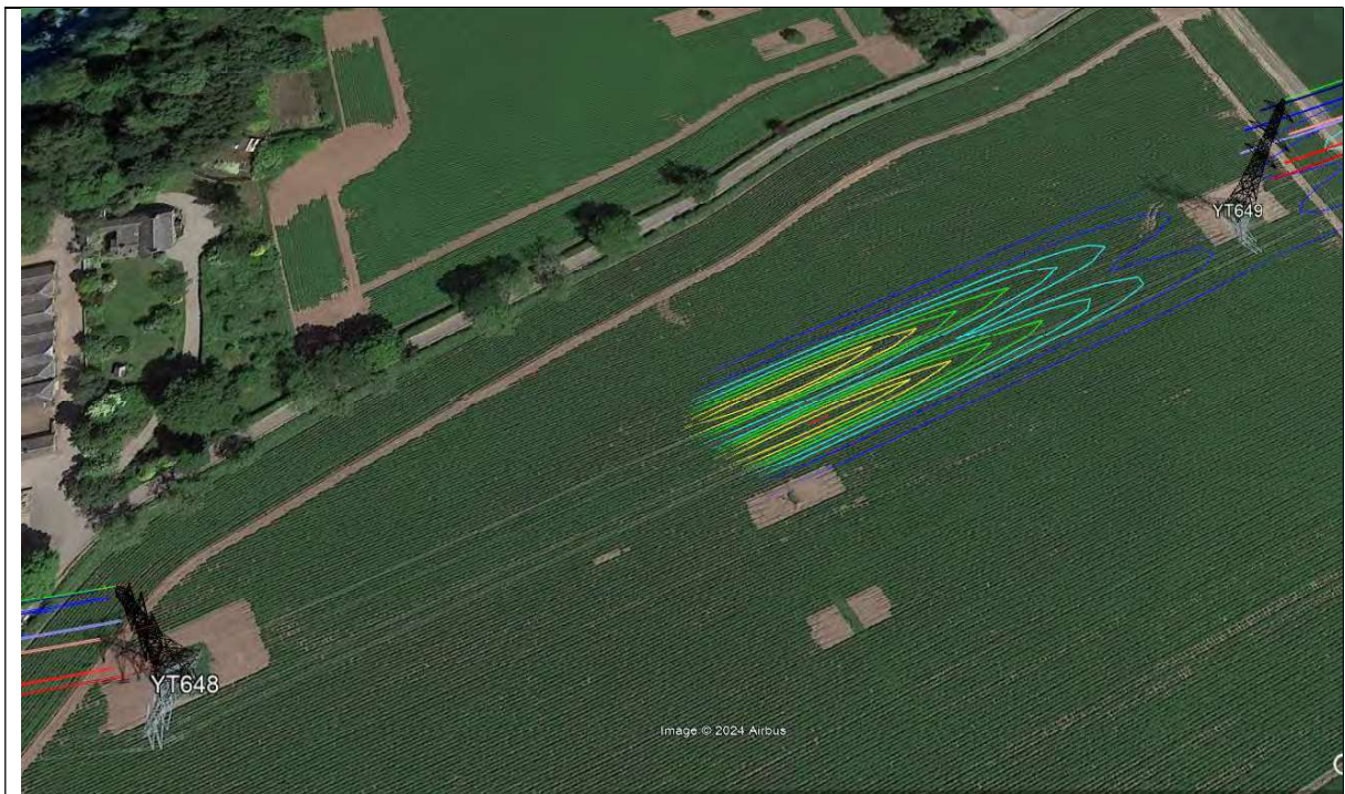
Figure 5 Electric Field Contours (kV/m) for span 648 to 649
