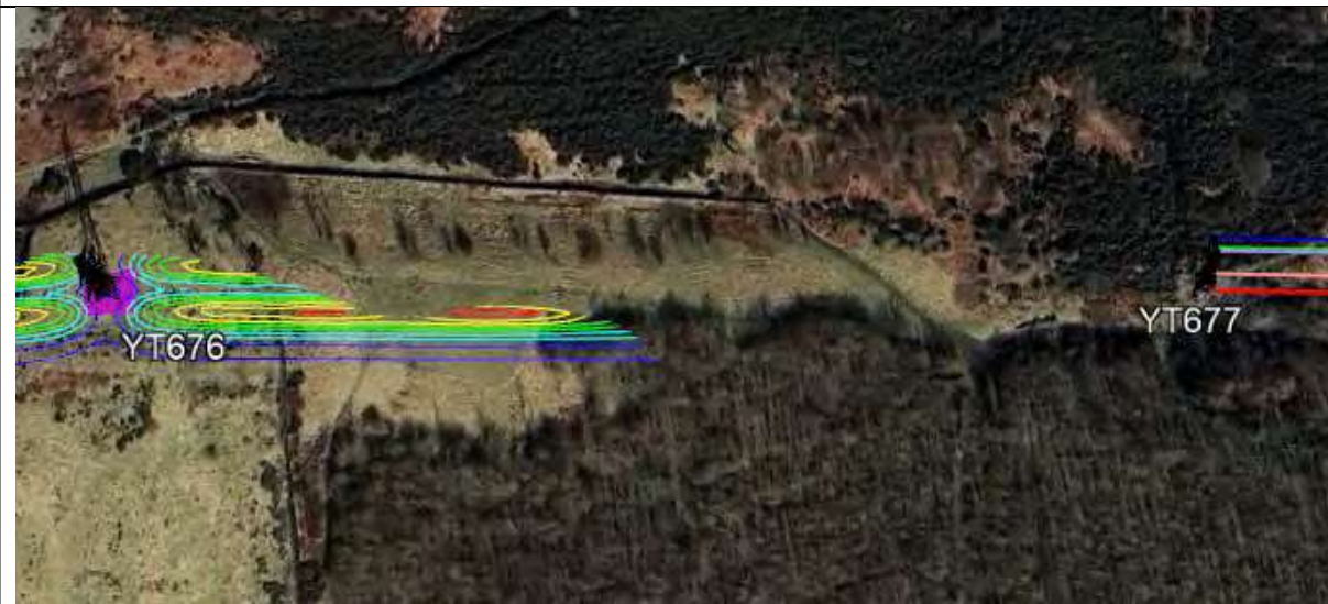
Figure 11 Electric Field Contours (kV/m) for span 676 to 677
