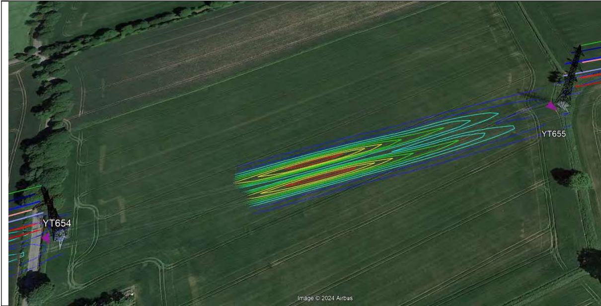
Figure 6 Electric Field Contours (kV/m) for span 654 to 655
