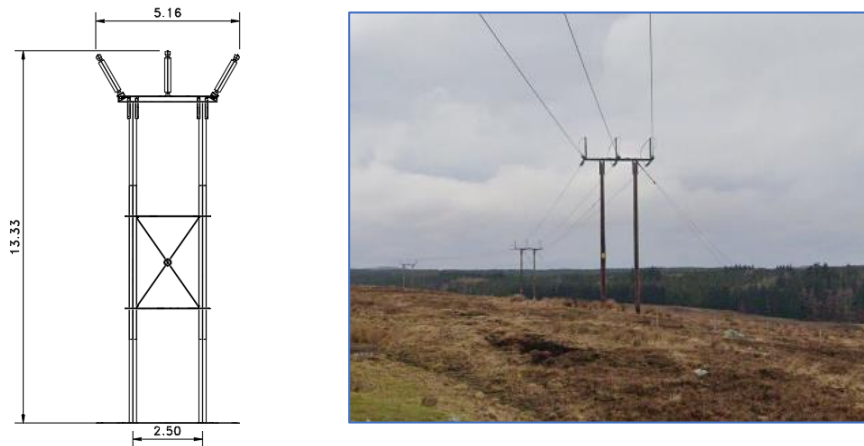
Plate 3.2: Proposed Trident H-wood poles Typical Schematic and Example Photograph
