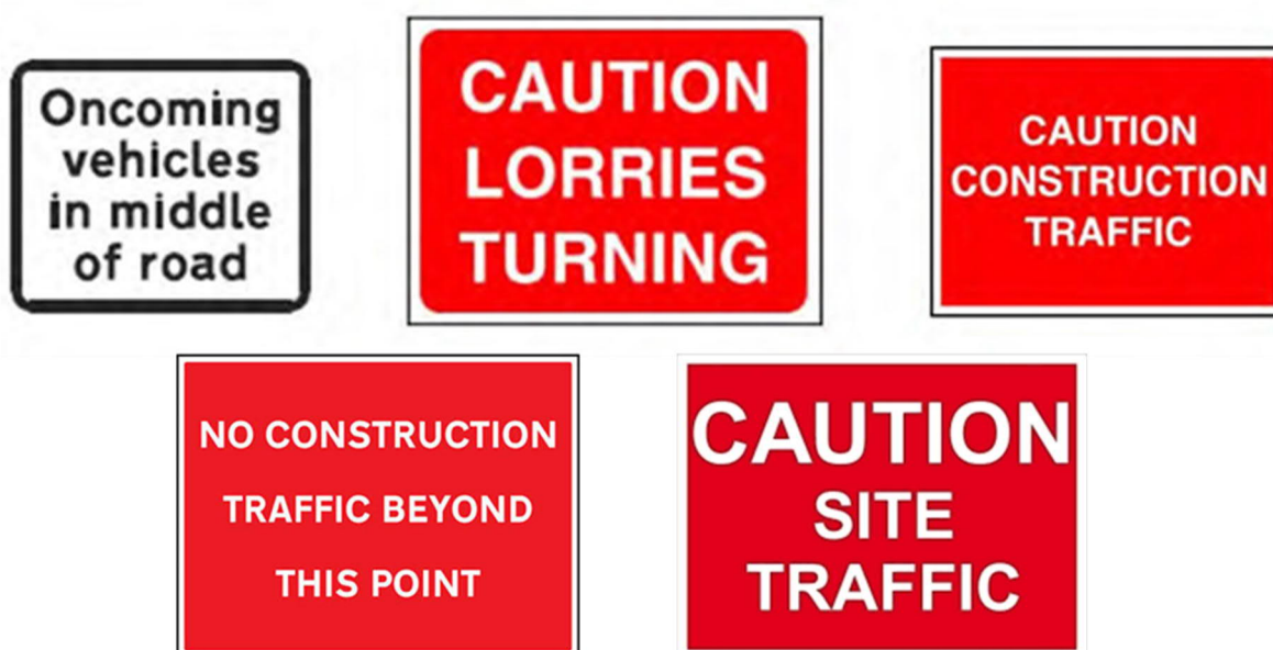
Figure 1 - Typical Advance Warning Signage
