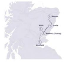
To facilitate this, we are proposing to establish a new 400 kV OHL between Kintore and Tealing. This requires two new 400 kV substations to be constructed, one at Fetteresso Forest (Hurlie), and one at Tealing, (Emmock), to enable future connections and export routes to areas of demand.
