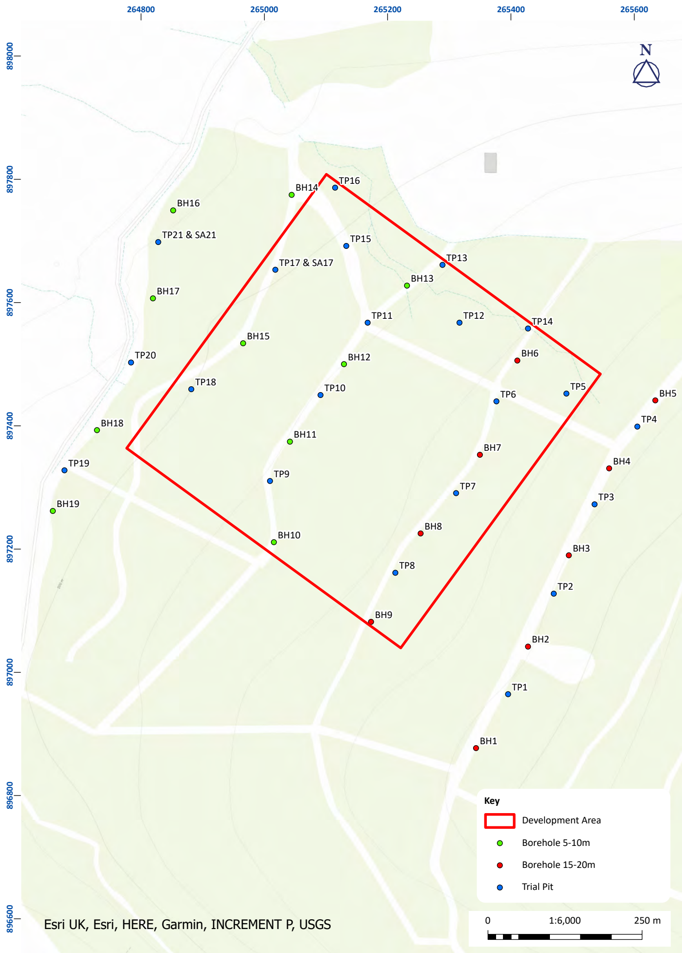
Figure 2: Watching Brief area showing borehole and trial pit locations
