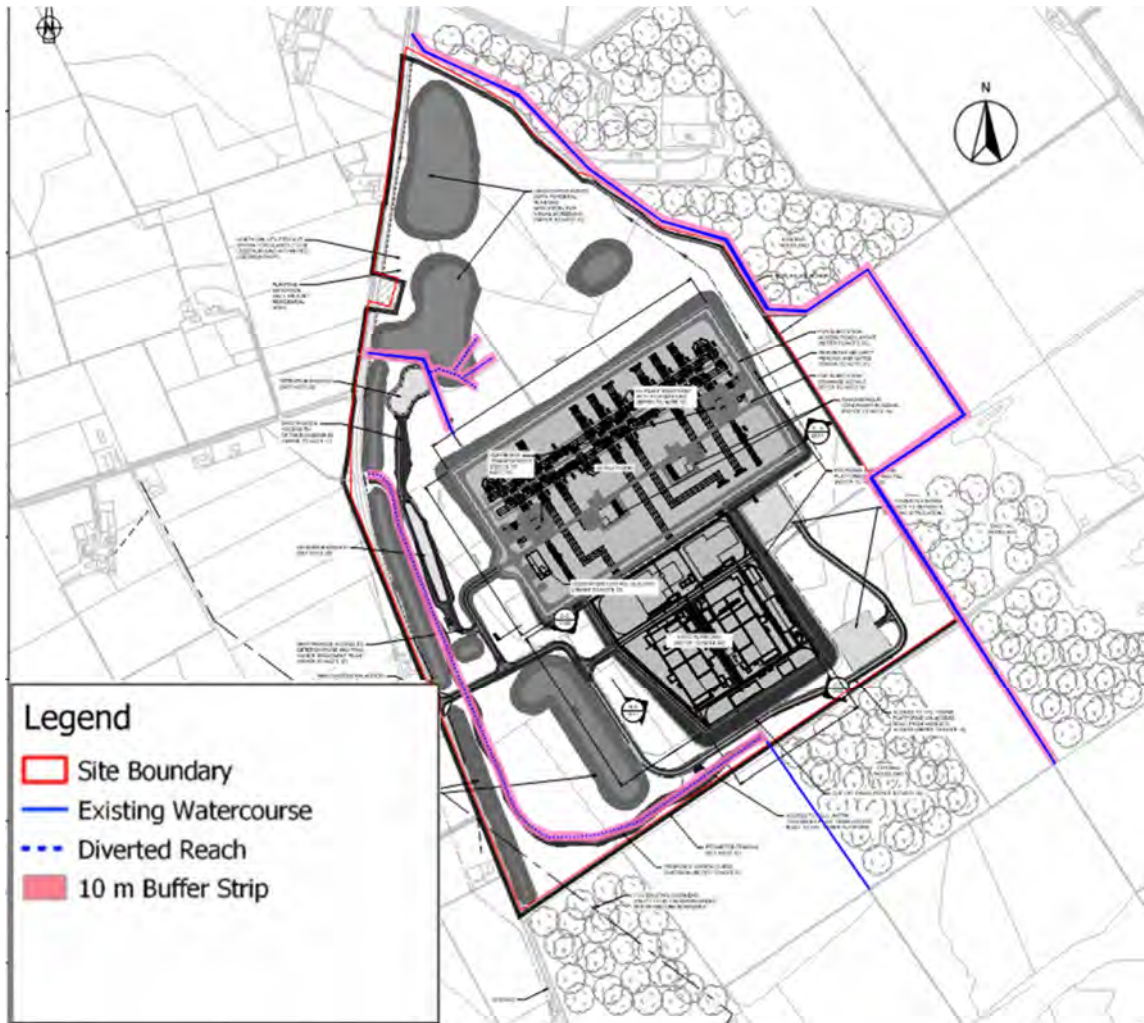
Figure 12: Location Plan Showing the Proposed Permanent Development Overlain with Watercourse Diversion Proposals.
