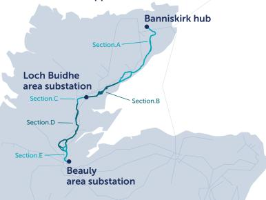
To support the growth in renewable developments across the north of Scotland, investment in our network infrastructure is needed to connect this power and transport it to areas of demand. This includes a new 400kV overhead line between Spittal and Beauly connecting into new substations near Spittal (Banniskirk Hub), Loch Buidhe (Carnaig) and Beauly (Fanellan).
