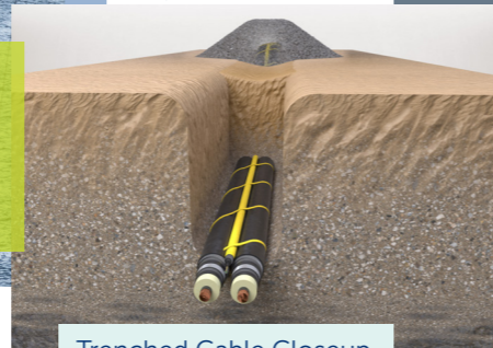
Trenched Cable Closeup.
