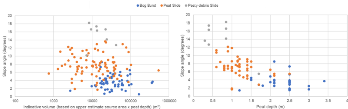
Plate 2.2 Reported slope angles and peat depths associated with peat slides and bog bursts (from literature review of locations, depths and slope angles, after Mills, 2002)
